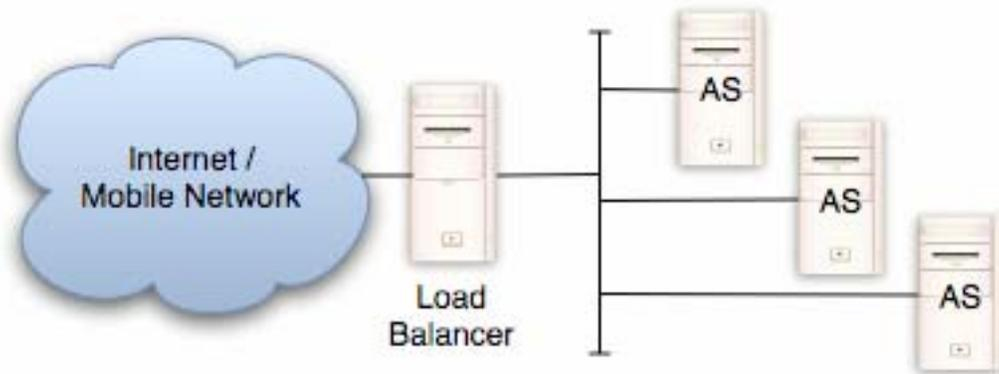
Figure 1: Clustered Load Balancing
